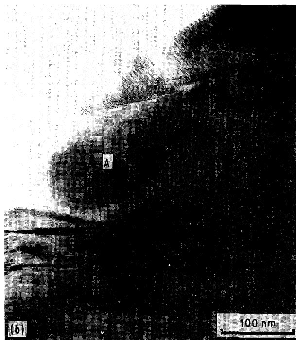
Figure 5 Transmission electron micrographs for hot-pressed samples (a) before annealing and (b) after annealing at 700 °C in air for 50 h.
